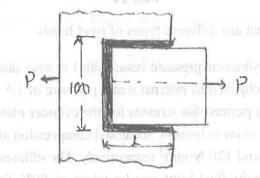
The strength of the welded joint should the equal to the strength of the plates to be joined. The permissible tensile and shear stresses for the weld material and the plates are 70 and 50 N/mm<sup>2</sup> respectively. Find the length of each parallel fillet weld.
